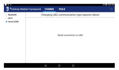
Once the tablet is powered back on, swipe down from the top of the screen again to confirm you see "LMU is Connected." If it still states "LMU is Disconnected," please contact Support for further assistance.
