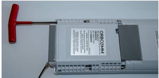
2. Pull apart the two pieces, and collect the two nuts. Place the two nuts in a safe place so they are not lost.
