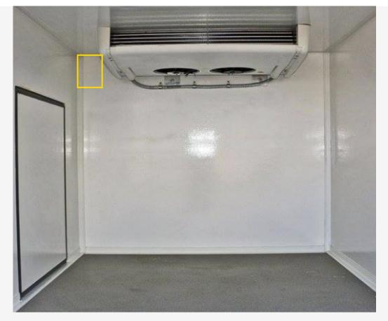
2. Identify a cable route from the temperature sensor location to the GPSI-3900. The cable placement should not prevent the use or removal of asset panels and should not leave the cable open to damage.
