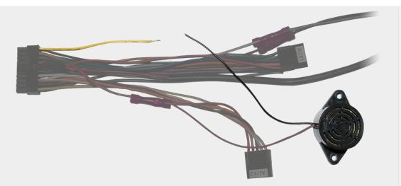
b. Using a butt connector, secure the buzzer's solid black wire to the solid yellow wire on the 20-pin harness.
