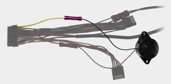
3. Secure the buzzer to the wiring harness using a zip tie.
