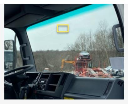
• Type 4: Angled/Split Windshield; Right windshield, down ~4-6" down from roof and ~1"in right of the center divider.
