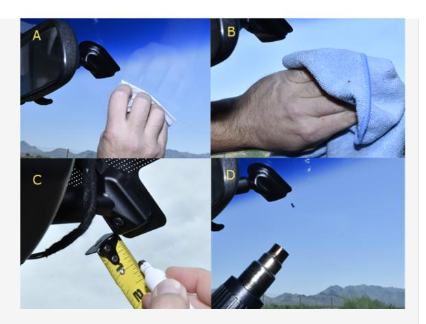
**Note.** Excessive heat may cause delamination of the windshield or cracking. Continuously move heat gun to not apply heat in one area for too long.
