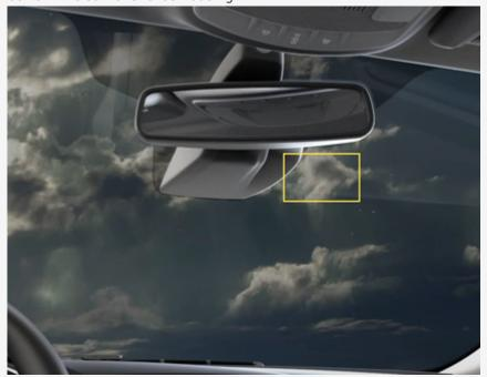
• Type 3: Without Rear View Mirror; Top center, ~4-6"in. down and 6"in. right of center windshield.
