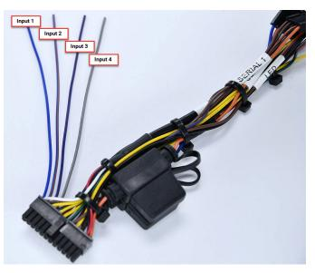
**Note.** Input 1 is a 12 VDC (+) input, used only in light-duty vehicles (e.g., F150-F550, Chevy 1500-3500, etc.). If you have a 24 VDC (+) system or a heavy-duty Class 6,7 or 8 vehicle, you must use one of the three negative (-) inputs (Input 2, 3 or 4). For negative inputs, in-cab switches typically sense a change in voltage from 0-12 VDC (+), so you may need to reverse the polarity by installing a relay. (See below)
